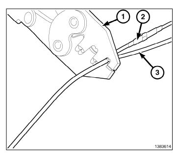
15. Solder (3) the connection (2) together using rosin core solder (1).
